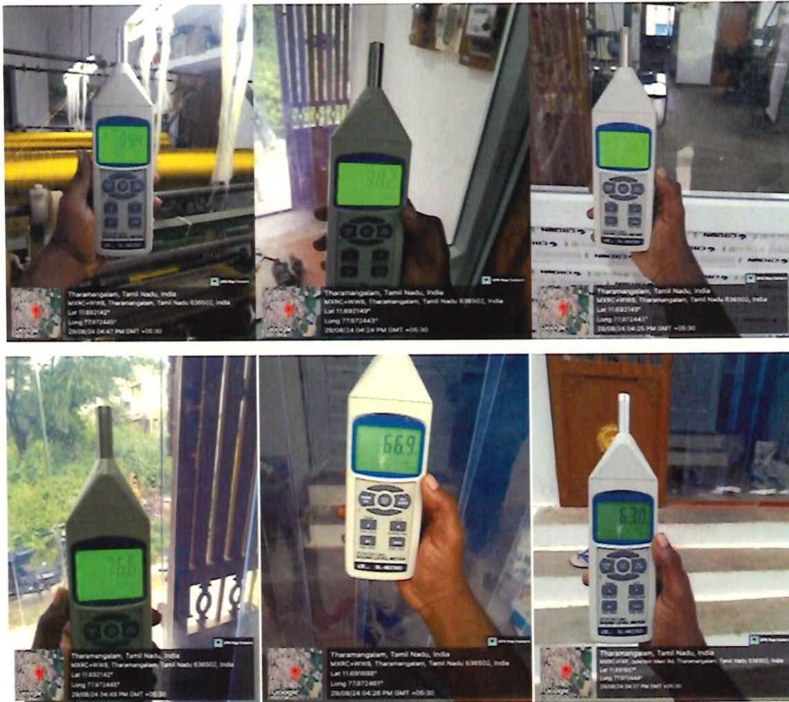
Figure 4.13: Noise level after installation of noise control measures along the transmission path (i) at loom [99.4 dB(A)] (ii) before UPVC door [98.2 dB(A)] (iii) behind UPVC door [76.7 dB(A)], (iv) before PVC curtain [76.6 dB(A)], (v) behind PVC curtain [66.9 dB(A)], (vi) behind gate [63.0 dB(A)]
